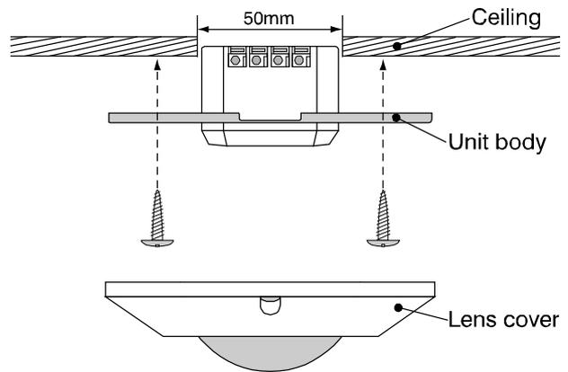
1. Please refer to the "DETECTION PATTERN" and locate the position where sensor can cover all routes of movement.
