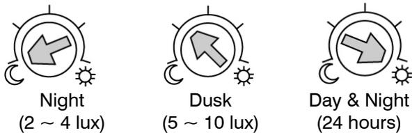
**NOTE: If multiple sensors are installed in the same area to control different lighting, and LUX of each sensor is individually set, the brightness of the **first** switched on light may disable the other sensors.**
