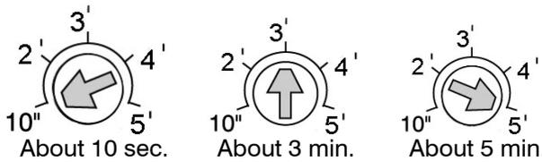
**NOTE: Any further movement detection before the delay time expired will reset the timer.**
